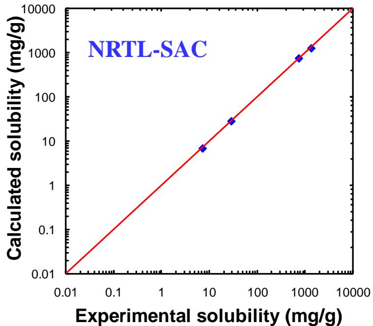
Solubility of co-crystal formers in 4-5 solvents was measured. Solubility in other solvents was then calculated from NRTL-SAC model with ASPEN software. Values given are for L-Tartaric Acid.
